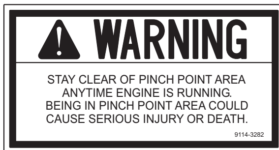
Located on right and left rear frame, hydraulic reservoir & boom head P/N 9114-3282
